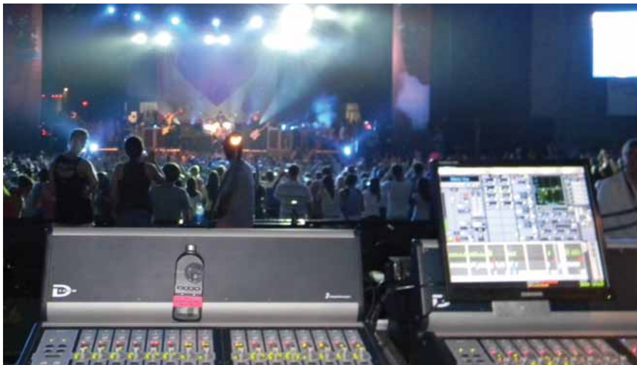
FOH during Boys Like Girls, headlining the Bamboozle Road Show 2010. The best seats in the house for sound. Note the Radio Shack sound level meter with the red tape on the mixer board. This sound level meter showed 104 dBA in this photo.
