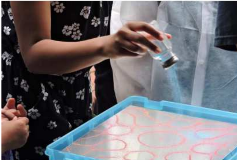
A Chladni Plate (sound resonance demonstration) was used to engage with Philadelphia Science Festival attendees by showing that sound is a physical energy that can be explored visually.
